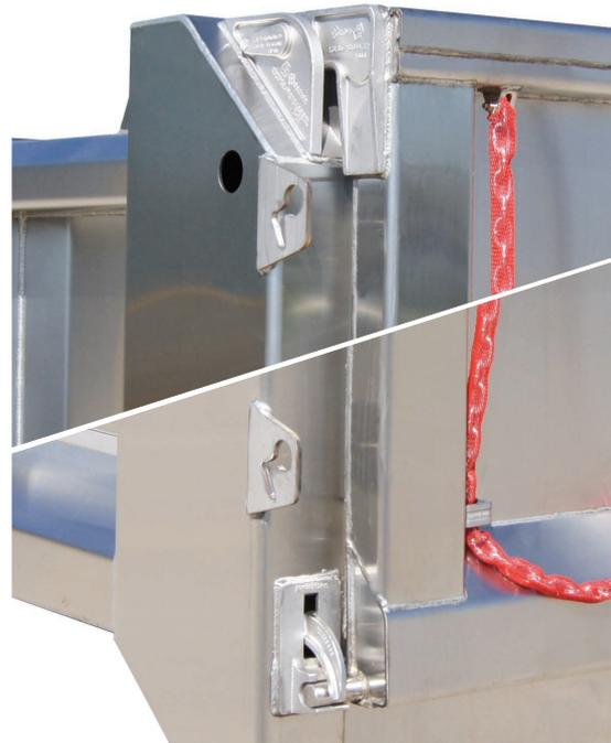
Pictured is a close view of the tarp friendly stainless upper hardware and the stainless lower latching hardware standard on the 453U
