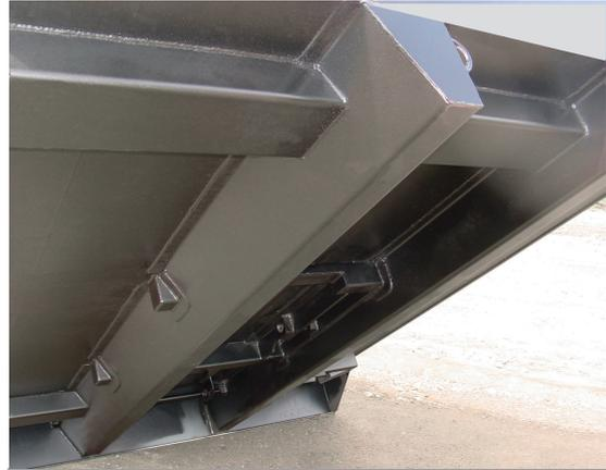
A bottom view of the 453U reveals the cross-memberless understructure with heated body option
