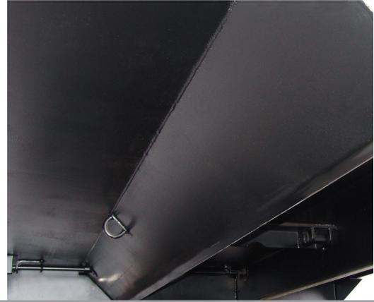
The crossmemberless understructure of the 530U and 533U bodies use 3/16" X 100K formed 10" formed trapezoidal longbeams.
